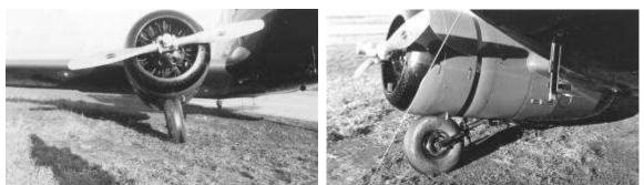
T-50 with collapsed gear (four photos) Kansas City, 1938 (Mort Brown, Photographer)
