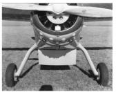
Cessna C-38 with wide landing gear & belly flap
